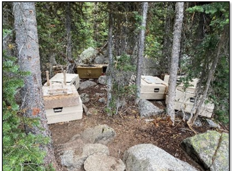
Figure 2. Vault Toilet boxes from Alpine Lakes Wilderness, full of human waste, awaiting air transport for removal Photo by Chris Armatas
